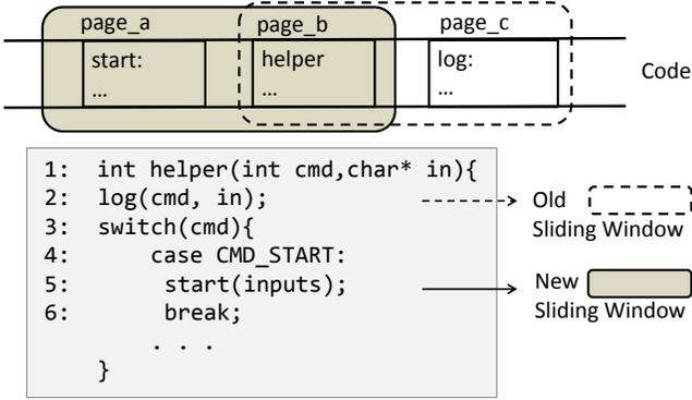
Fig. 2. **The sliding window and its update.** In this example, the size of the sliding window is 2 pages. When the execution flow reaches to *log* function (line 2), the sliding window is (*page\_b*, *page\_c*). Later the window is updated to (*page\_a*, *page\_b*) when the *start* function (line 5) is executed. Note that the code pages in the sliding window can be non-contiguous.
