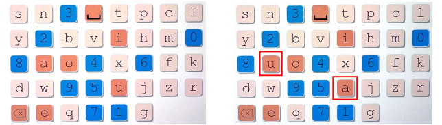
(a) Private keyboard composed by an app's secure endpoint (b) Refreshed keyboard with letter swapping after 'a' is clicked.
