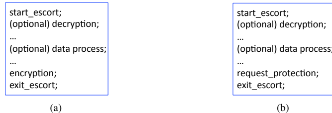
Fig. 4. The two types of PCB format. (a) A PCB ending with encryption. Thus, the hypervisor does not need to enforce access control on the data; (b) A PCB ending with protection requirement. Therefore, the hypervisor must enforce access control on the data to restrict the access.
