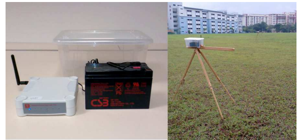
Fig. 1. Wireless router and accessories used in the testbed. Left: One node is composed of one Compex WP54G router, one 12V rechargeable lead battery and one plastic container to protect the hardware from rain. Right: Actual deployment of the node in the test site.
