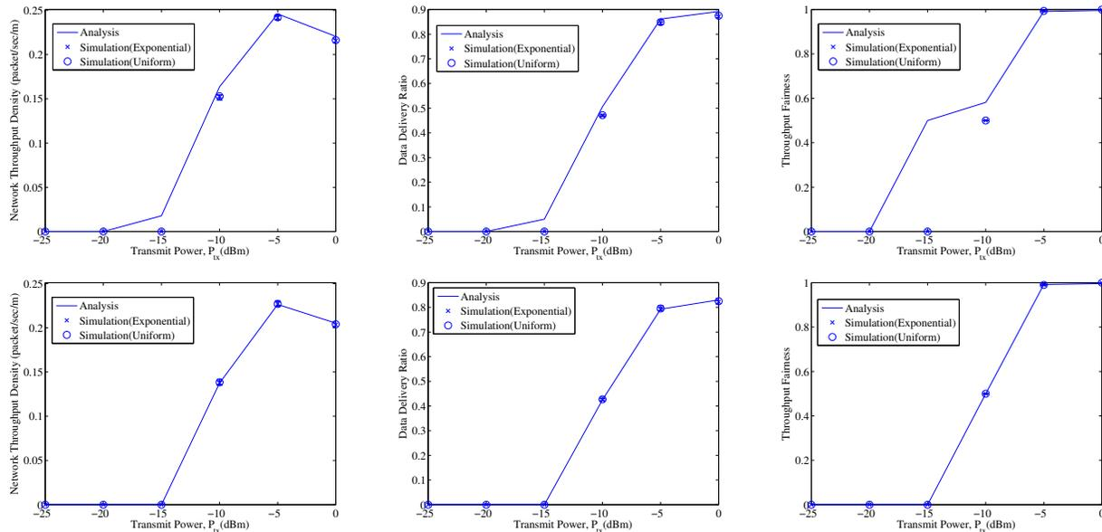
Figure 4. Network throughput density (left), data delivery ratio (centre) and fairness (right) vs transmit power for a 5-hop WSN-HEAP for railroad track monitoring with  $\theta = 5\text{dB}$  (top) and  $7\text{dB}$  (bottom).
