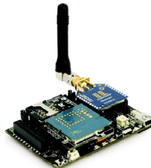
(b) Wasp mote sensor node with XBee-802.15.4
