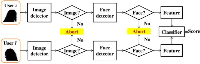
**Figure 4: The workflow of face recognition for identity linkage.** A face detector is employed to extract the face from a pair of profile images. Then a pre-trained face classifier outputs a confidence score in  $[0, 1]$  indicating how likely the two faces belong to one person.
