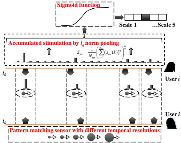
**Figure 6: Multi-resolution temporal behavior modeling.** A set of pattern-matching sensors are designed. For two users, sensors are used to detect the corresponding type of matched behavior within certain temporal scales. When all the matched behaviors have been detected by sensors, an  $l_q$  norm pooling and nonlinear sigmoid mapping then aggregates all matched behavior signals into a multi-resolution similarity vector.
