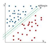
Figure 1: Maximum-Margin Hyperplane Calculated by SVM in Two-Dimensional Space
