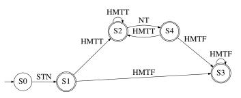
Fig. 4: StringTokenizer's Ground Truth Model. "STN": StringTokenizer(). "HMTT": hasMoreTokens() = true. "HMTF": hasMoreTokens() = false. "NT": nextToken().
