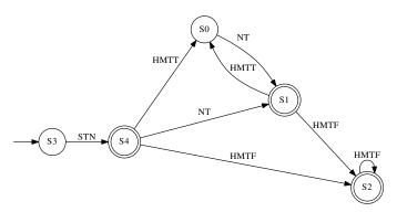
Fig. 3: StringTokenizer's SpecForge Model. "STN": StringTokenizer(). "HMTT": hasMoreTokens() = true. "HMTF": hasMoreTokens() = false. "NT": nextToken().
